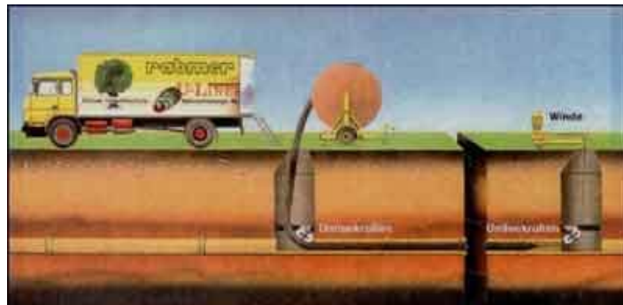
Figure 2. Technology Close Fit (Source: Rabmer)
