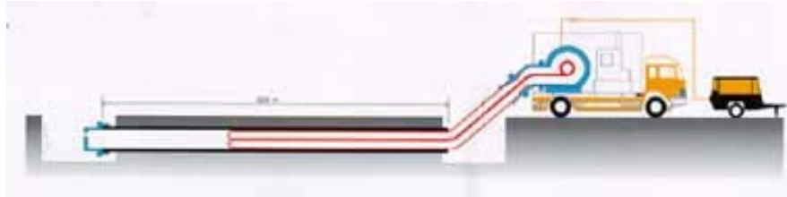
Figure 10: Schematically draft of an Inliner installation (Source: Rabmer)
