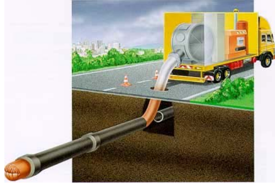
Figure 9: Inliner System (Source: Rabmer)
