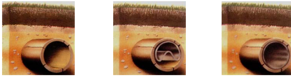
Figure 5-7: “Old pipe” / close fit liner before reformation / close fit liner after reformation (Source: Rabmer)
