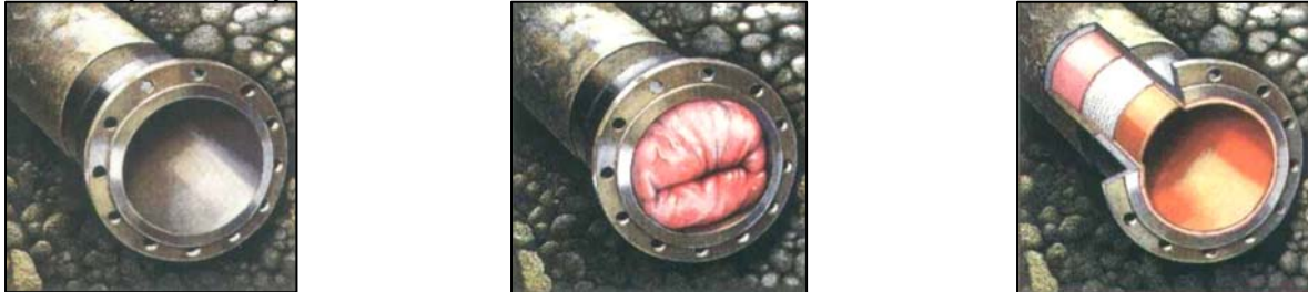
Figure 11 – 13: Pipe before rehabilitation / pipe with impregnated textile tube before heating / rehabilitated pipe
